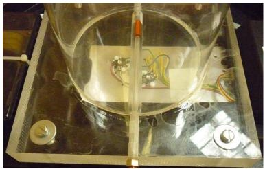
4. Attach the cloudy plastic pipe to the blue valve on the Ball-Bubble Tube column.
